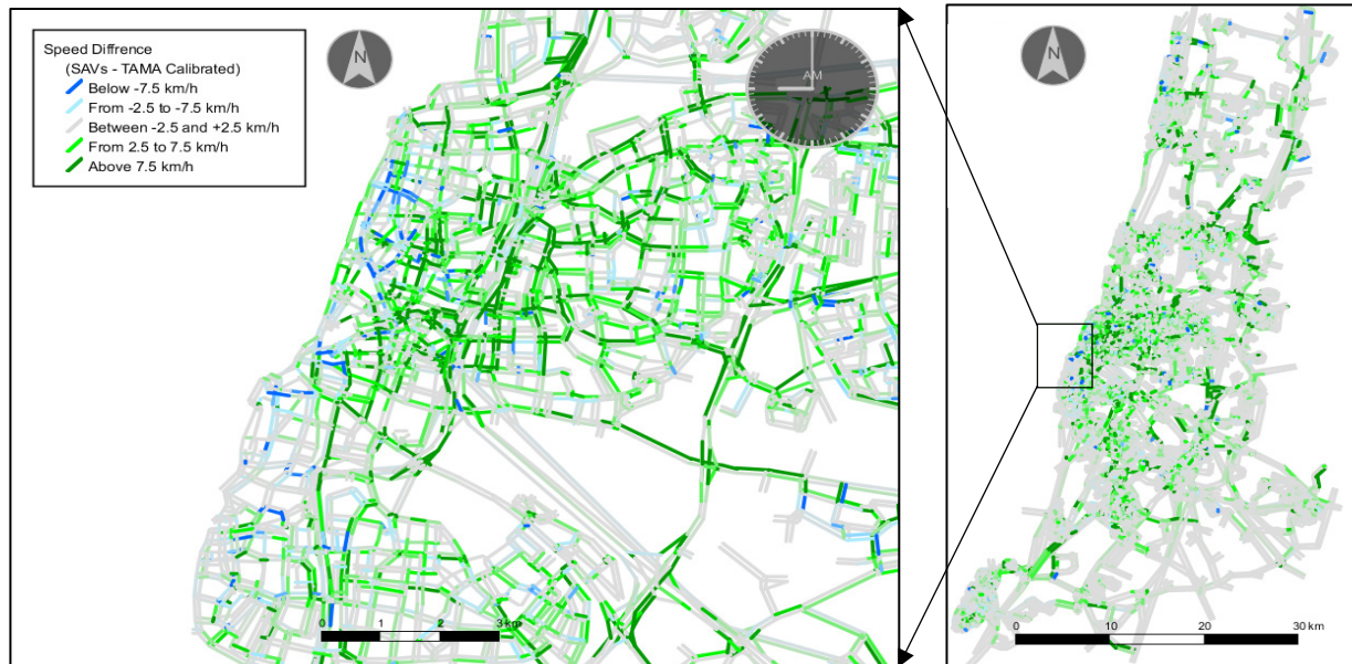
Figure 5. Average Speed Difference between 100K SAVs with 4 seats and calibrated TAMA simulation (08:00-09:00)
