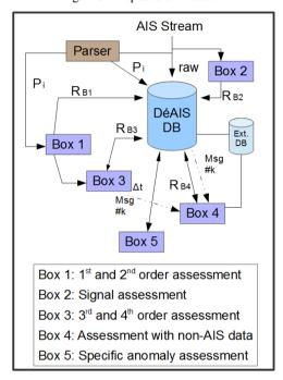
The signal is then parsed, and the parameters of those messages, that is the data within the data fields, are processed using the method for integrity assessment presented in section 3.2. This method takes place in box 1 (for first and second levels) and in box 3 (for third and fourth levels).
