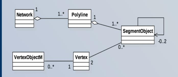
Polylines are decomposed into segment lines in order to be edited individually if necessary.
