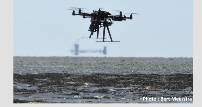
With an Unmanned Airborne Vehicle or drone, photos are taken of the mussel bed and computed into an ortho-photo with a detail of 2 cm. Current legislation limits the operation area for drone flying to 500 meters from the take-off point. To map a mussel bed longer then 1000 meters requires multiple take-off locations. Images with a detail of 1 mm can be acquired by flying at an altitude of 5 meters above ground level. This method is used to sample selected parts of the mussel bed.
