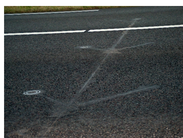
Figure 2: Road Temperature sensor. The sensors are on the car lanes.
