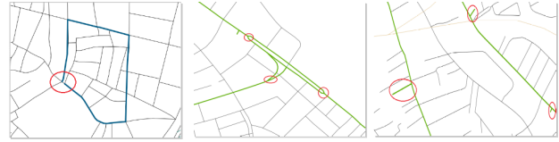
Figure 5: Main errors in polygon geometry and topology: holes, duplicated geometries, dangle edges
