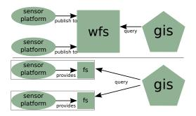
Figure 1: *Top*: each sensor platform publishes to an OGCcompliant Web Feature Service. *Bottom*: each sensor platform implements a feature service
