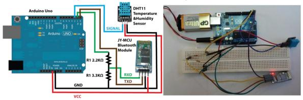
Figure 2: ArdSense module, left: schematic, right: real circuit.
