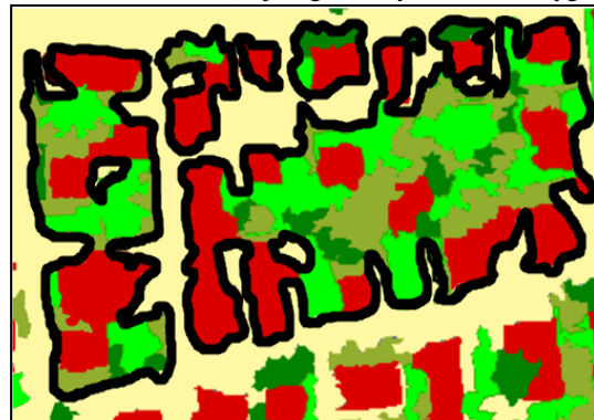
Figure 4: In this example the Object Grouping function constructs one cluster (object geometry is a MultiPolygon)
