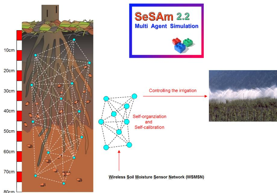
**Figure 1:** Physical construction of the wireless soil moisture sensor network.
