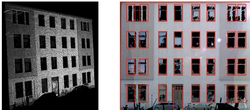
Figure 8: Point cloud of a facade and the reconstruction result visualized in the orthophoto.
