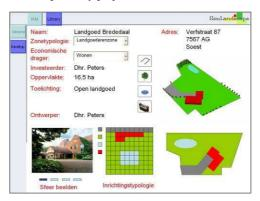
Figure 8: parcel-design editor for arranging lay-out components
